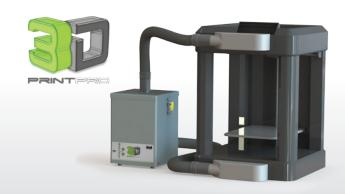
All units have HEPA grade particulate filter media which has an efficiency of 99.997% at 0.3µm, and deep bed activated carbon filters to remove organic gases and vapours.
