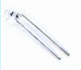
SP38.01 LOOSE L.E.D. CUT AND LEFT BEND
