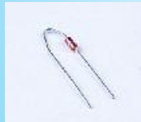
SP22.21 CUT AND BEND FOR VERTICAL MOUNT
