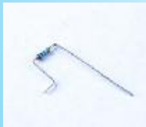
48.0L02.06 CUT AND "SEAGULL WINGS" FORM
