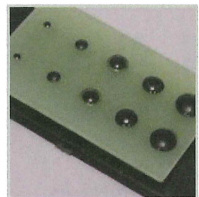
Caulking of fixing resin
